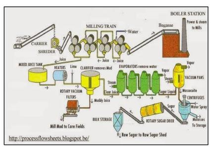
helps in extracting maximum sugarcane juice. The remaining solid fibrous material is known as bagasse.
