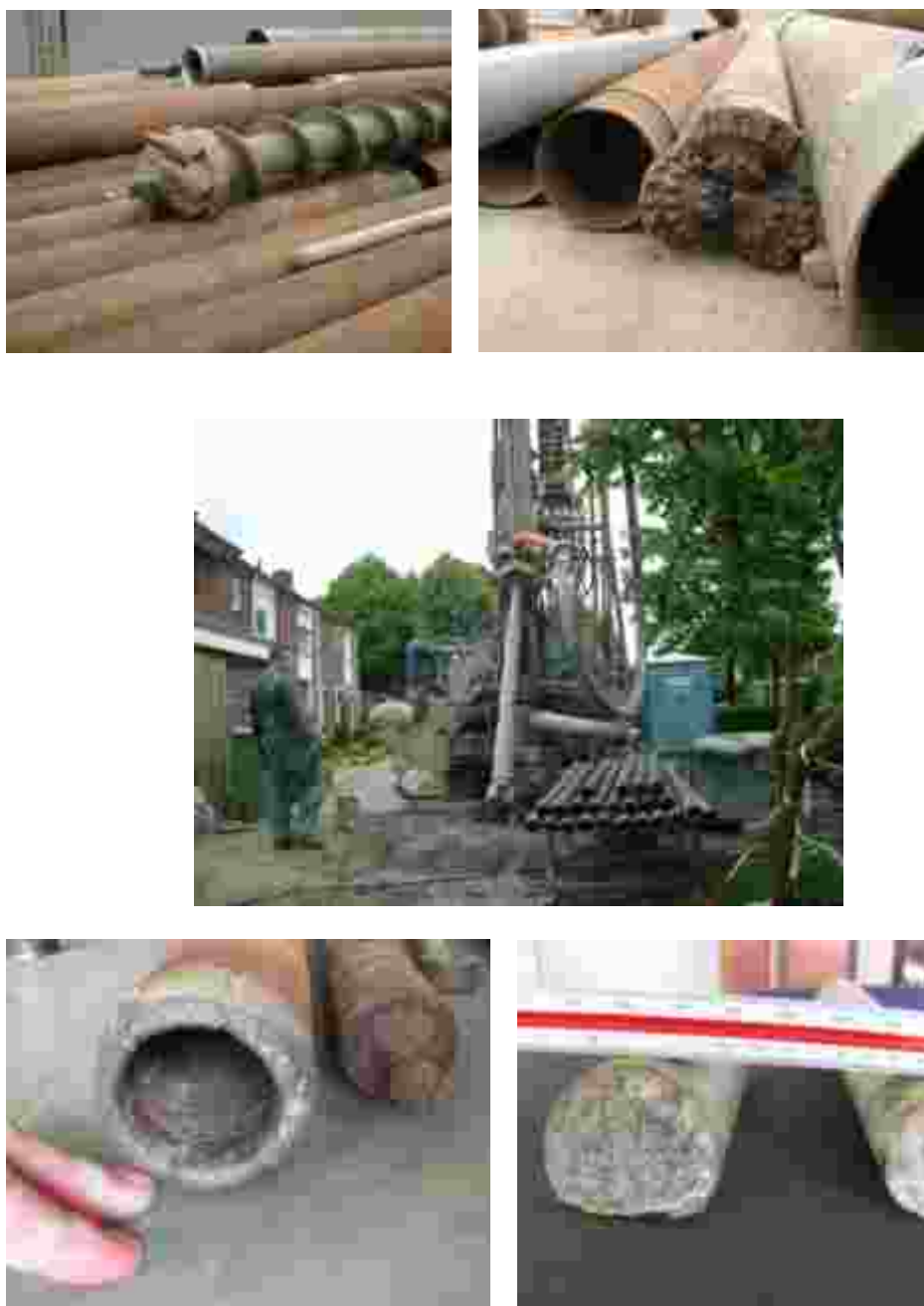
Figure III-2.2-iii. 13d-h: Examples of cased auger/pulse drill required for Hard ground and rock drilling
