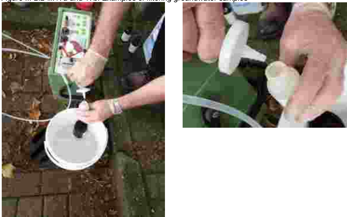
Figure III-2.2-iii.17a and 17b: Examples of filtering groundwater samples
