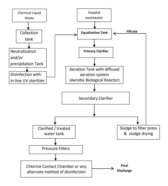
Figure 4: Scheme for Wastewater
