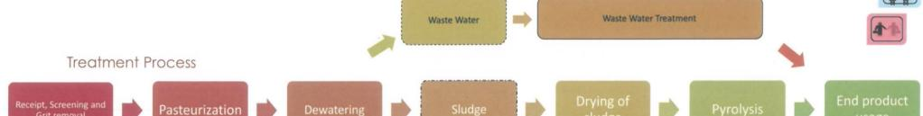
Faecal Sludge and Septage treatment process goes through 6 stages:
