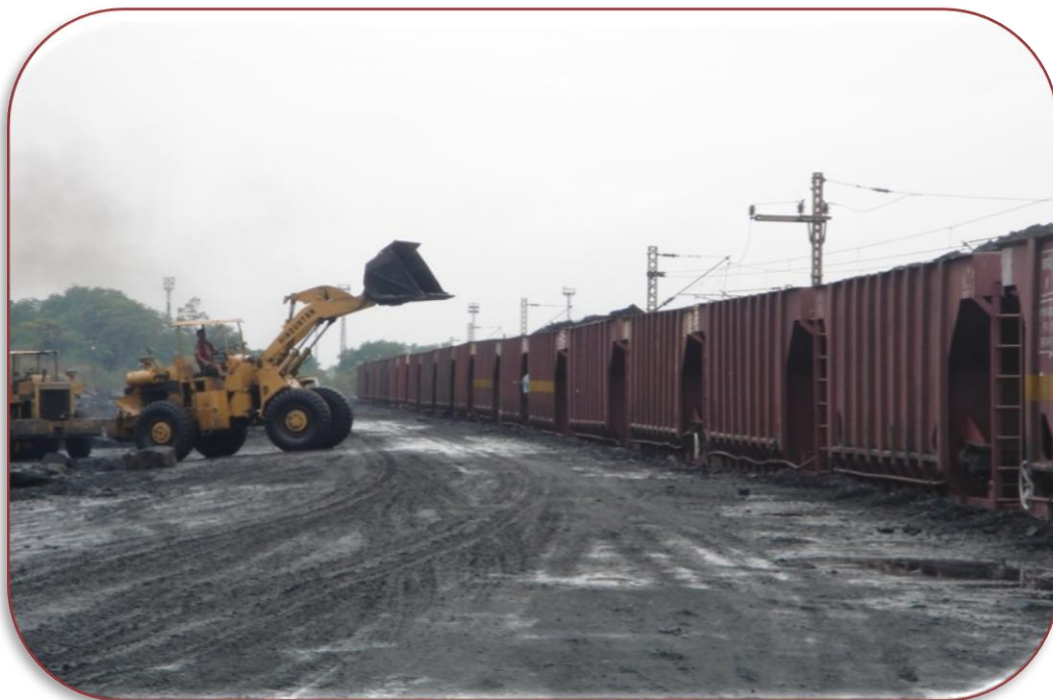
FIGURE 4.1 LOADING OF COAL THROUGH JCB
