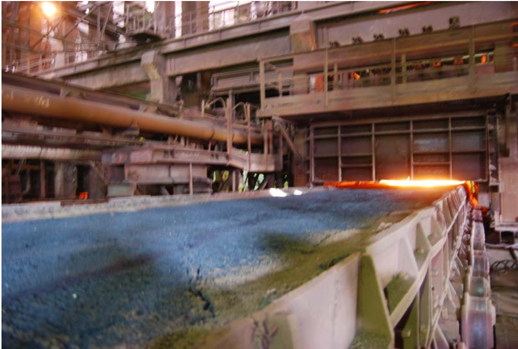
Fig. 3.9: Ignition of sinter mix in a sinter strand
