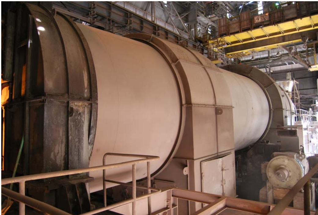
Fig. 3.8: A mixing and nodulising drum
