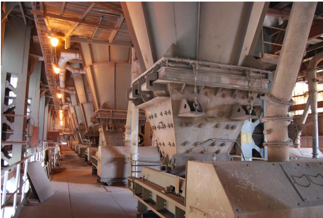
Fig. 3.7: A raw material proportioning section
