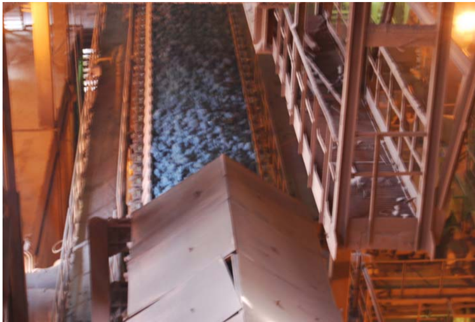
Fig. 3.11: A Straight line cooler
