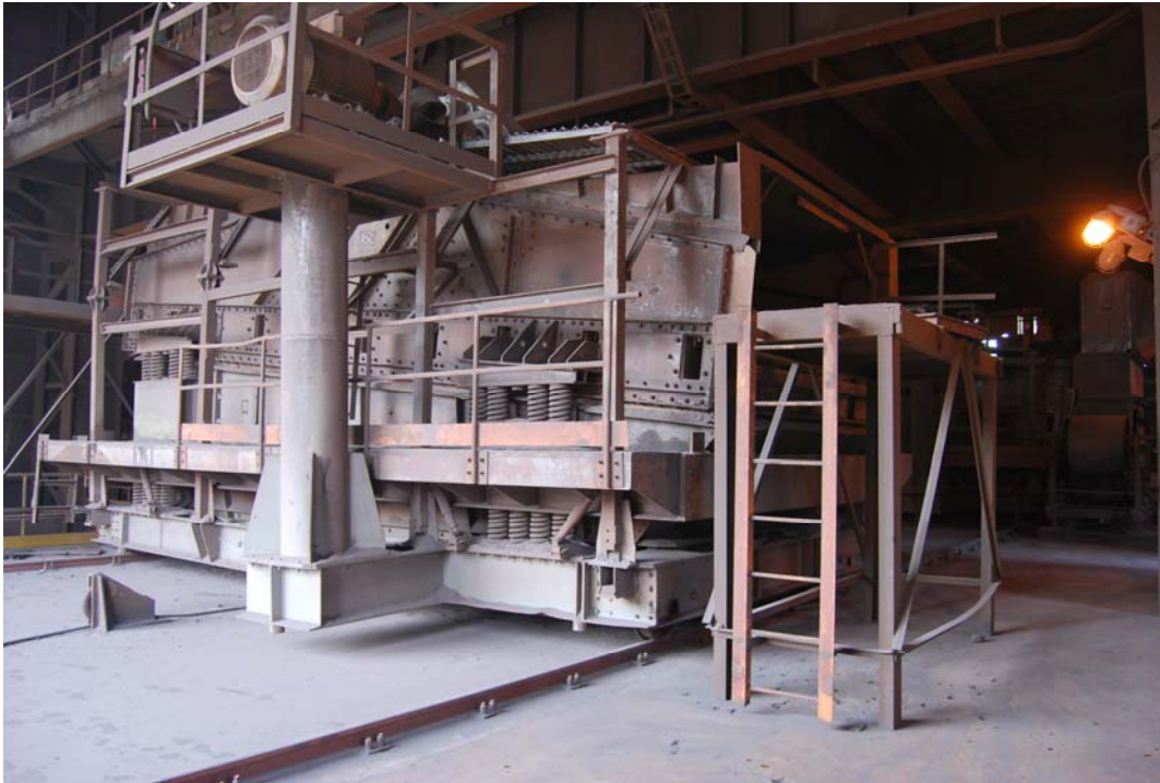
Fig. 3.13: Sinter Screening Machine
