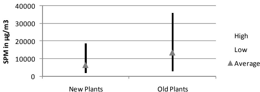
Fig. 5.9: Summarized fugitive emission monitoring results of RSPM
