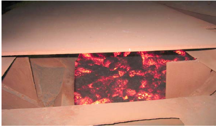
Fig. 3.10: Hot sinter at cooler feed end
