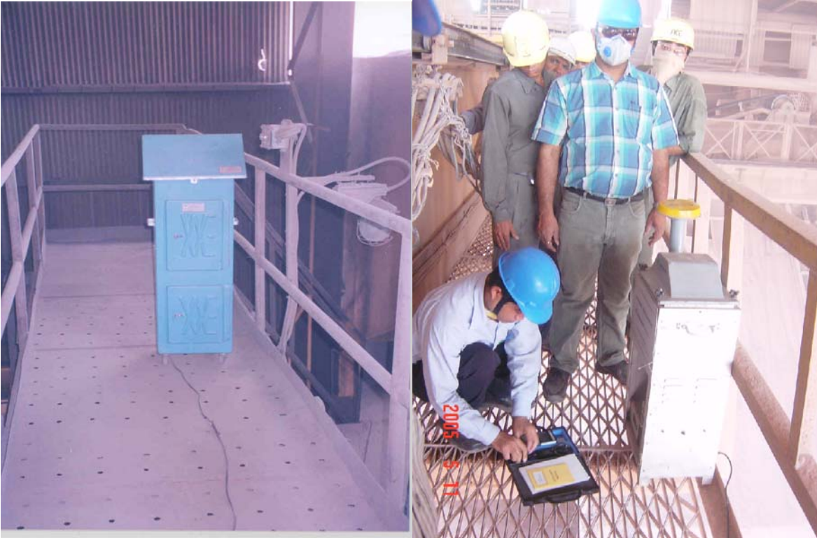
Photographs 6.1: showing HVS/RDS Monitoring in Progress
