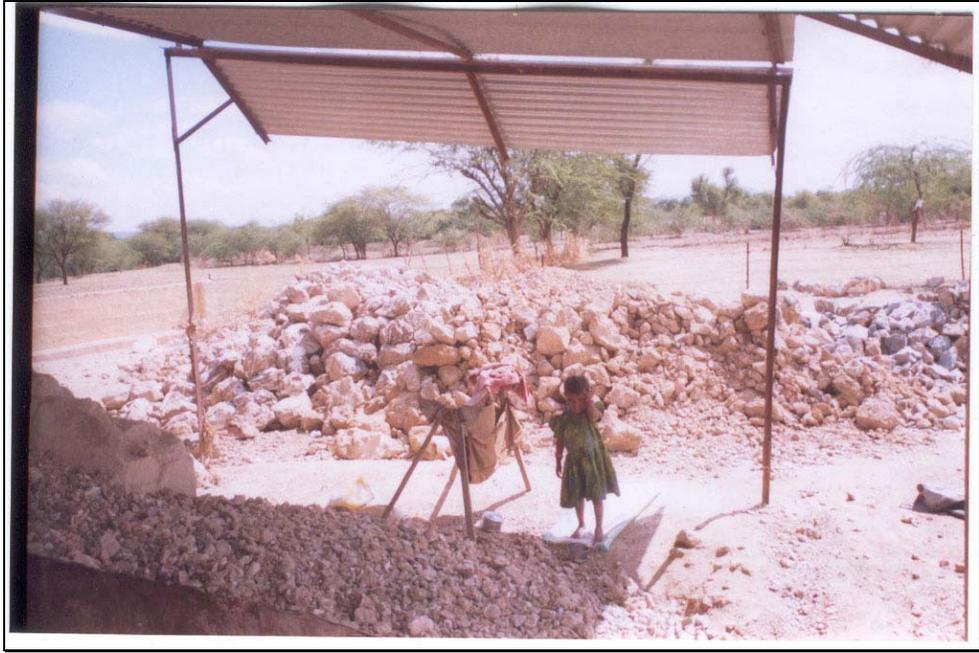
Picture 1: Showing asbestos-bearing stones spread open in an unorganized asbestos mill.
