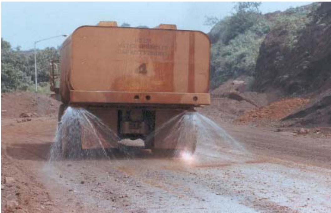
Fig. No.5.2.3.1 Haul Road Water Sprinkling System
