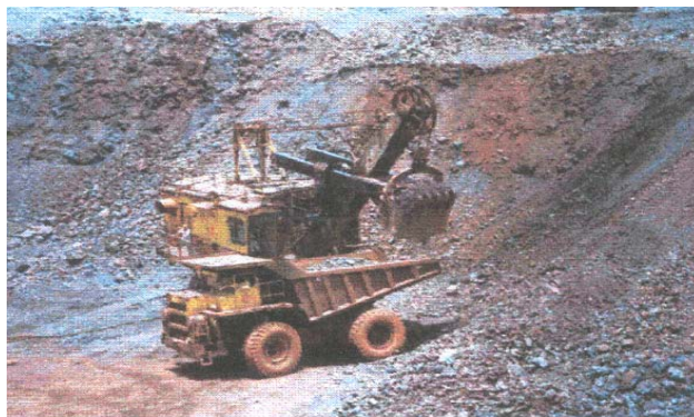
Mechanised mining operation by 4.6 m 3 Electric Rope Shovel with 50 T rear discharge Dumpers
