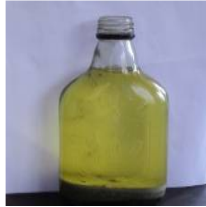
Leachate from unremediated soil
