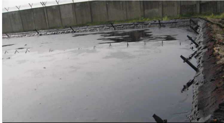
Oily sludge in being dumped in a pit in a Group Gathering Station of M/s ONGCL in Assam. Oily sludge is found stored in unlined or not properly lined pits.
