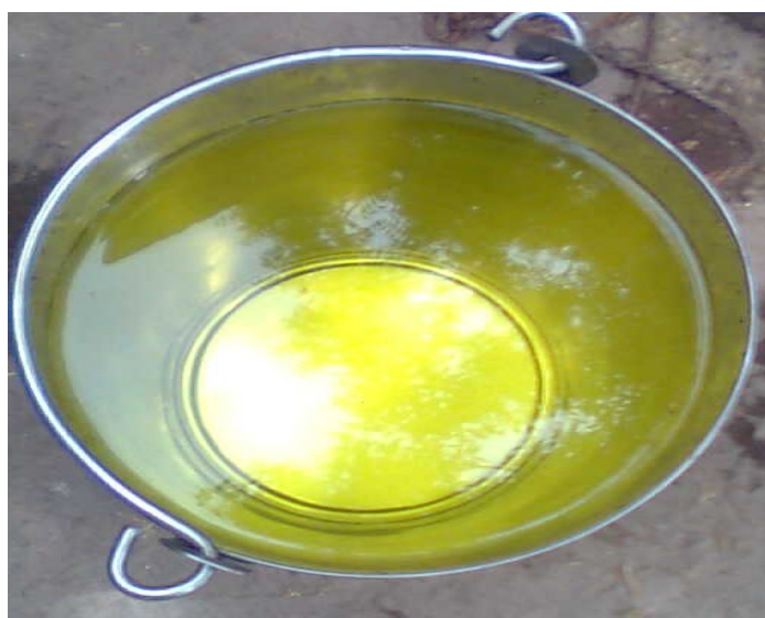
Figure 11.2 : Pale yellow colored Groundwater due to high Cr (VI) observed in Rania area
