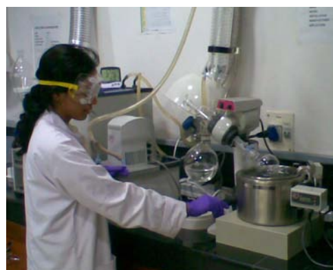
Figure 6.4 : Sample extraction and concentration for pesticides residues analysis in surface water samples
