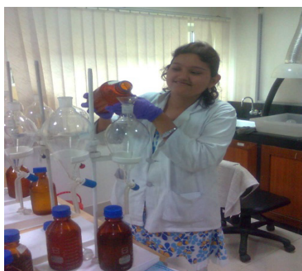
Figure 6.4 : Sample extraction and concentration for pesticides residues analysis in surface water samples
