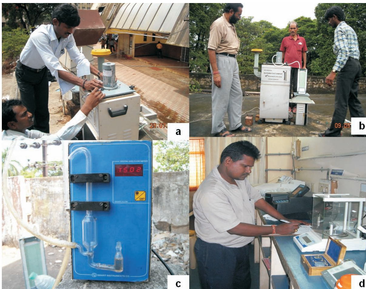
Figure 5.30 a. Field calibration b. Top loading calibration of Respirable Dust Sampler c. Use of dry gas meter for gaseous calibration d. Calibration of balance
