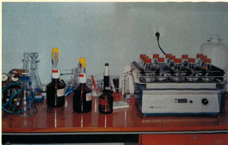
Figure: 4 Organic Halide Adsorption by Shaking Technique (Batch Method)
