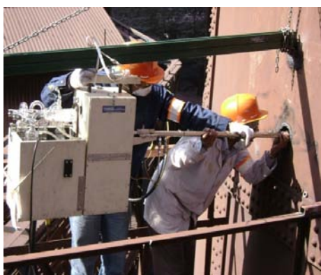
Sinter Plant Stack Emissions Monitoring
