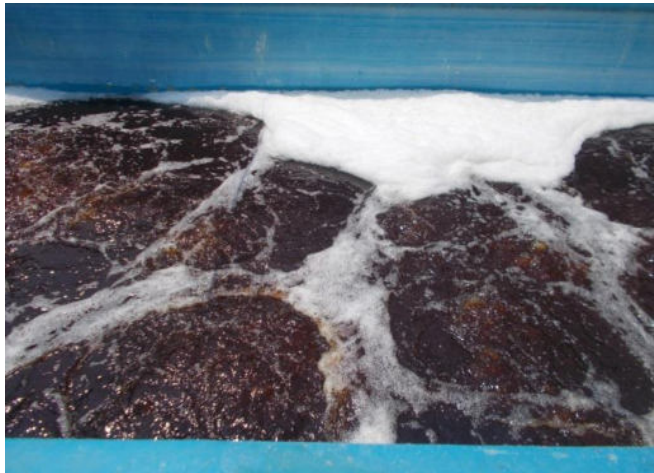
Storage of excess MVR concentrate
