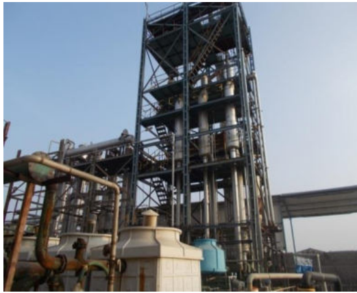
MEE with 3 effect forced circulation system Solar ponds for natural evaporation of concentrated effluent
