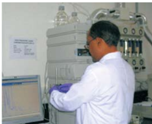
Figure 7.9 : Chlorobenzenes by High Performance Liquid Chromatograph (HPLC)
