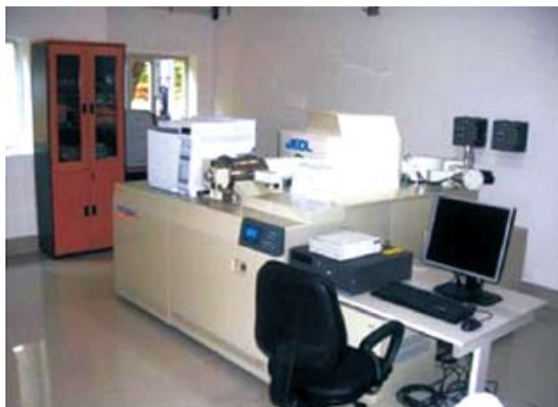
Figure 7.7 : High Resolution Chromatograph – High Resolution Mass Spectrometer for Dioxin / Furan Analysis
