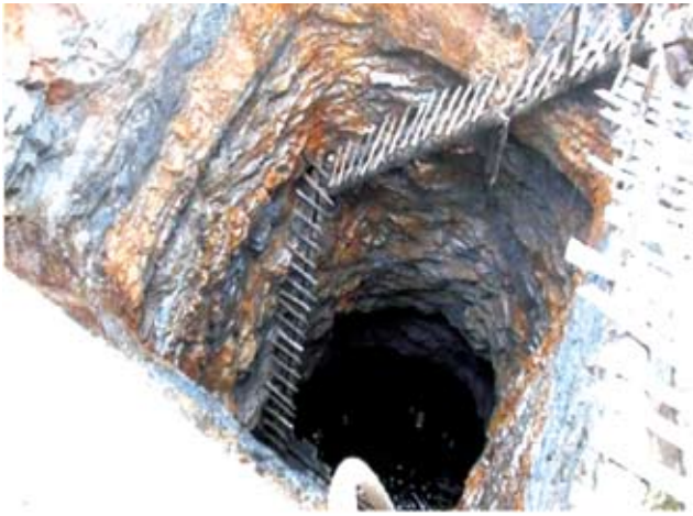
Box cutting Rat-hole mine
