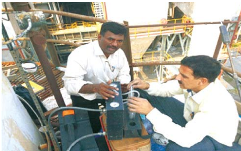
Monitoring of boiler stack at Waste to energy plant, Okhla
