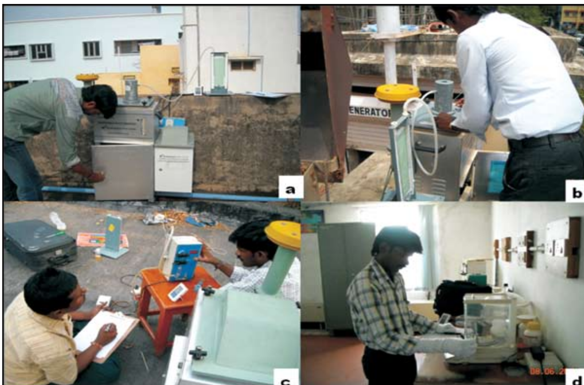
Plate I.2. Field calibration a, b. Top loading calibration of Respirable Dust Sampler at Kurnool and Goa c. Use of dry gas meter for gaseous calibration at Vizag d. Calibration of balance at Ramchandrapuram
