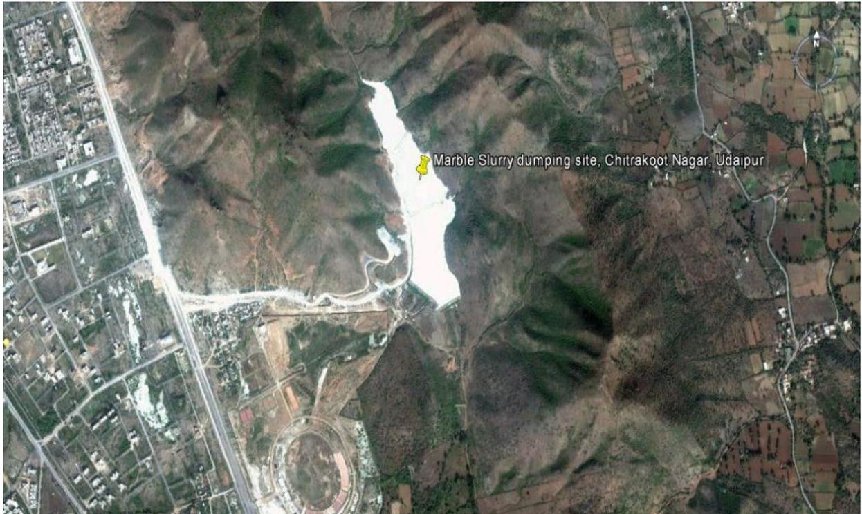
dumping/disposal is being done through tankers. This 30ft deep dumping yard needs to be raised upto 100fts high parapet walls to overcome the problem of slurry overflow during rainy season. Earlier the slurry was used to landfill the Khelgaon low-lying area.
