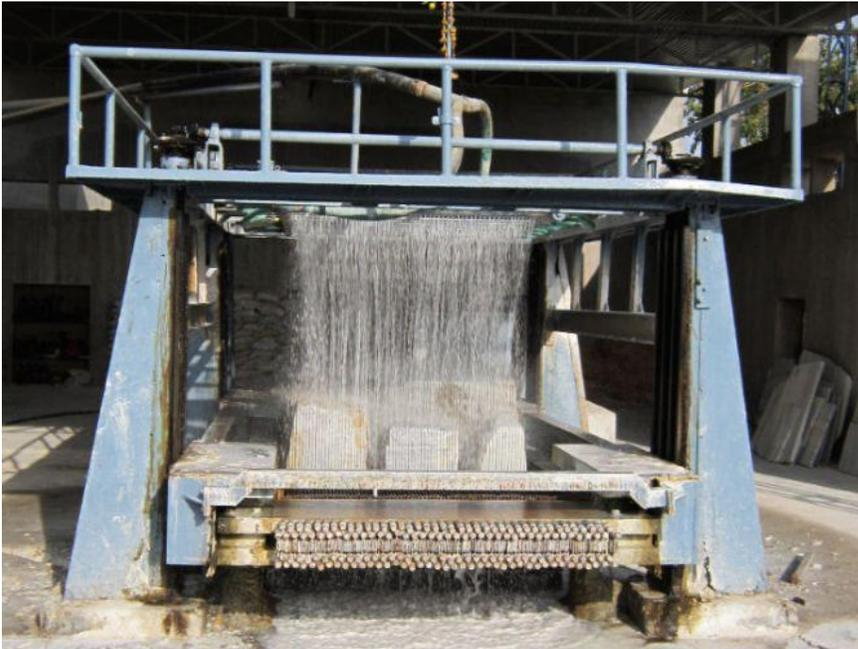
teeth and cut block into required thickness. The normal thickness is 15-20 mm. This thickness of segment is approx. 5mm while saw thickness is 3 mm. On one gang saw on an average 20-40 Tons of marble is processed daily. During operation water is being
