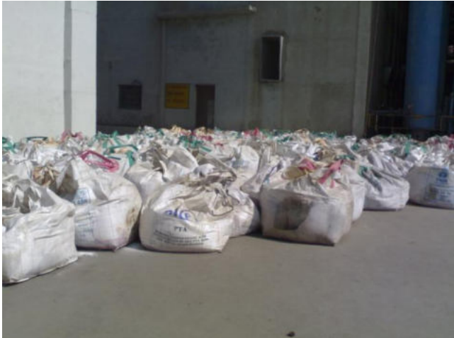
HW stored openly in HDPE bags
