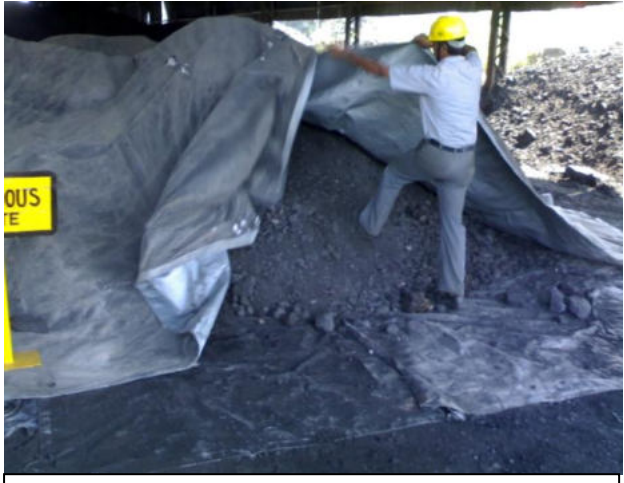
Tarpaulin sheet covered on the SPL
