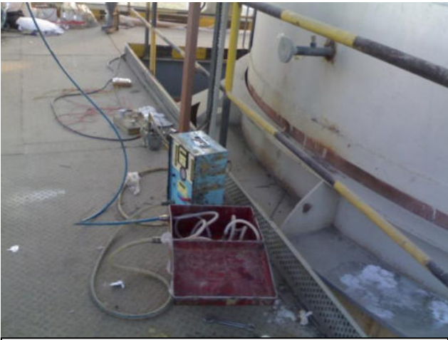
Stack monitoring during co-incineration
