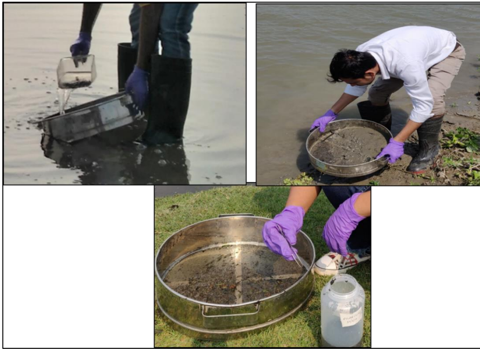
Fig.5. Collection of Macro-invertebrates in Substratum of Sand or Silt
