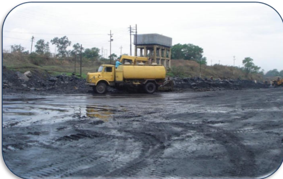
FIGURE 4.13 WATER TANKER FOR SUPPRESSION OF COAL DUST
