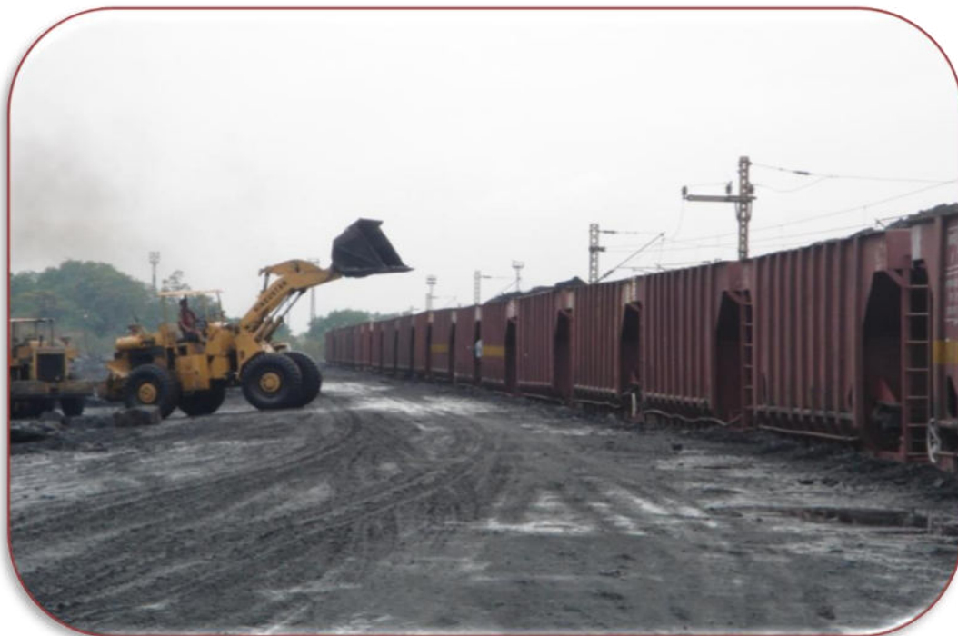
FIGURE 4.1 LOADING OF COAL THROUGH JCB
