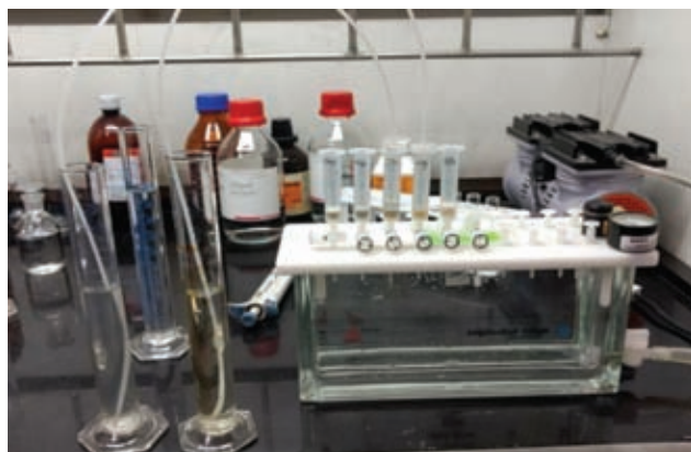
Solid Phase Extraction (SPE) of Wastewater Samples for PPCPs Analysis
