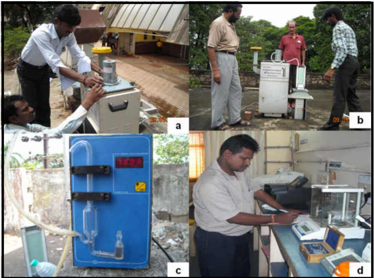
Plate 1.2. Field calibration a, b. Top loading calibration of Respirable Dust Sampler c. Use of dry gas meter for gaseous calibration d. Calibration of mettlet balance
