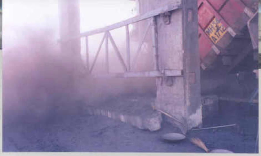
Photo 3.5 (a): Fugitive emissions from Coal Crushing Operation
