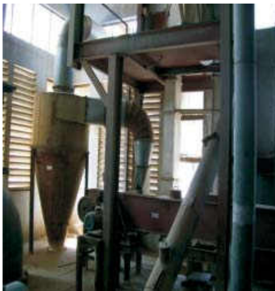
Fig. 4.4- Dust extracted through Cyclone
