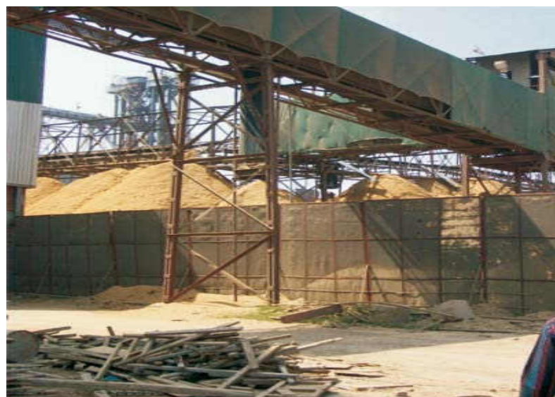
Fig 4.11-Husk Handling from storage yard to boiler using conveyor belts in large mills
