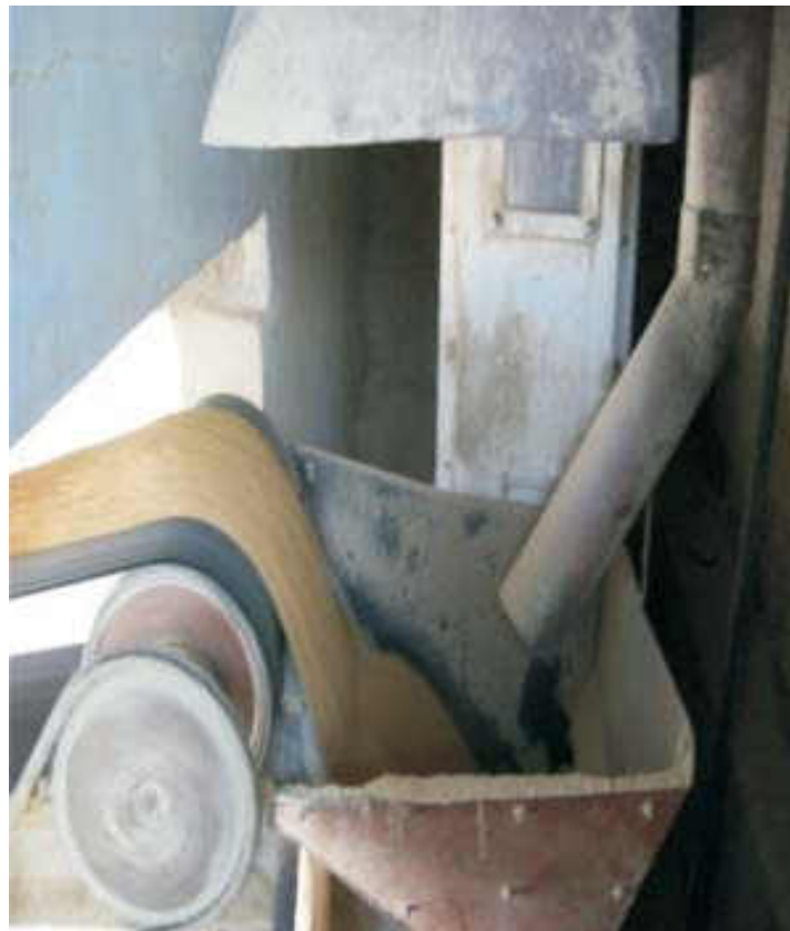
Fig 5.16-Extraction Hood near Bucket Elevator in large mills
