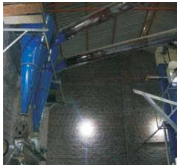
Fig 5.21-Suction ducts from polisher to cyclone for bran separation in small rice mills
