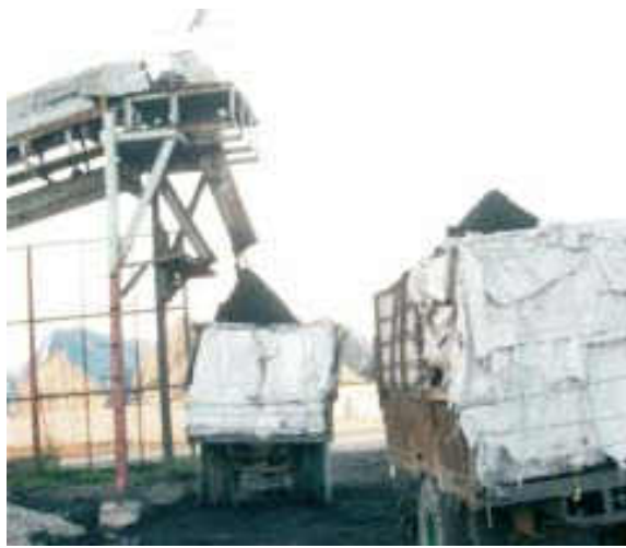
Fig 4.13-Mechanical handling of boiler ash
