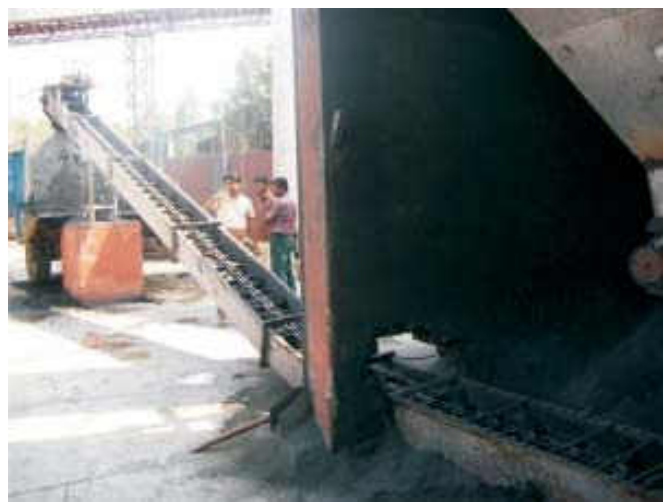
Fig 4.13-Mechanical handling of boiler ash
