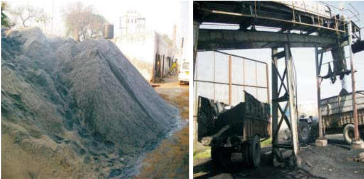
Fig 5.13-Fugitive Emissions from Boiler Ash temporary storage area
