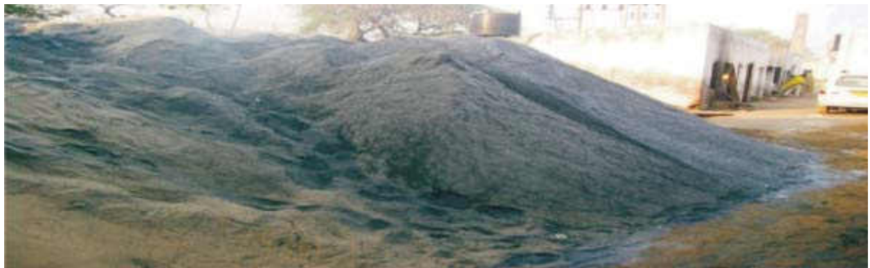
Fig 4.14-Open storage of husk fired boiler ash
