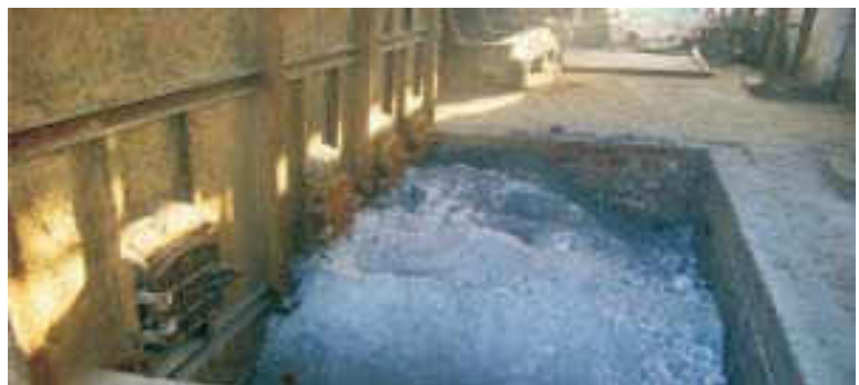
Fig 4.15-Partially covered storage of husk fired boiler ash
