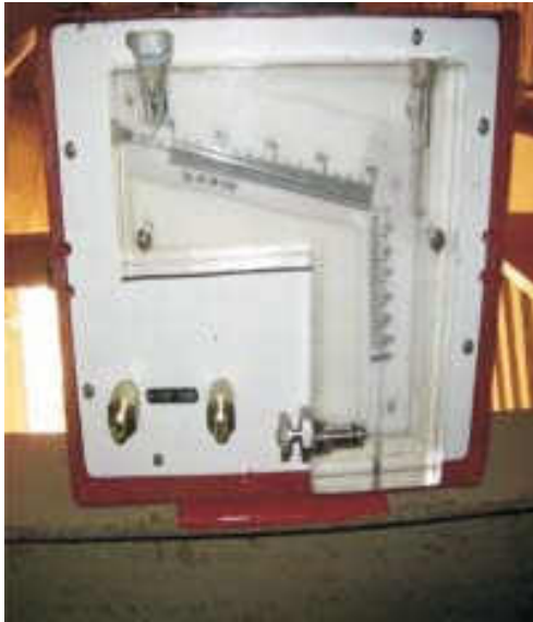
Fig. 6.1 Inclined Manometer used for Velocity Measurement
