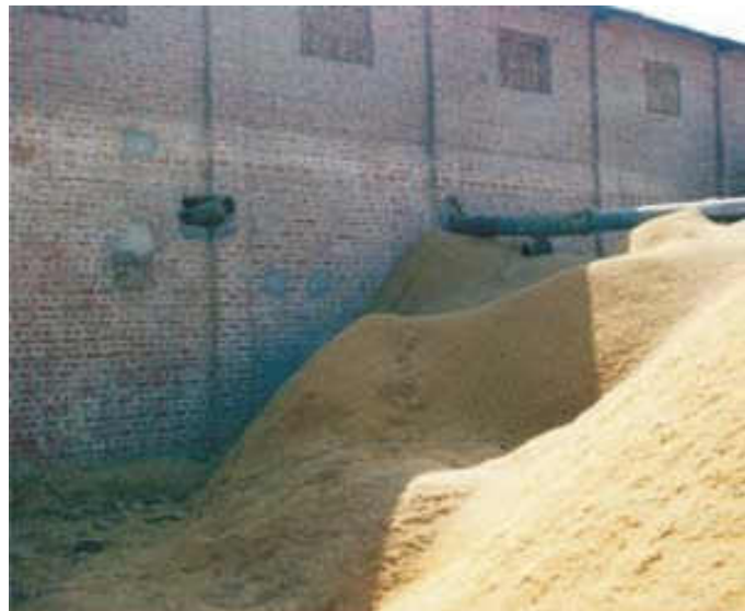
Fig 4.8-Fully open storage of rice husk without separating fines
