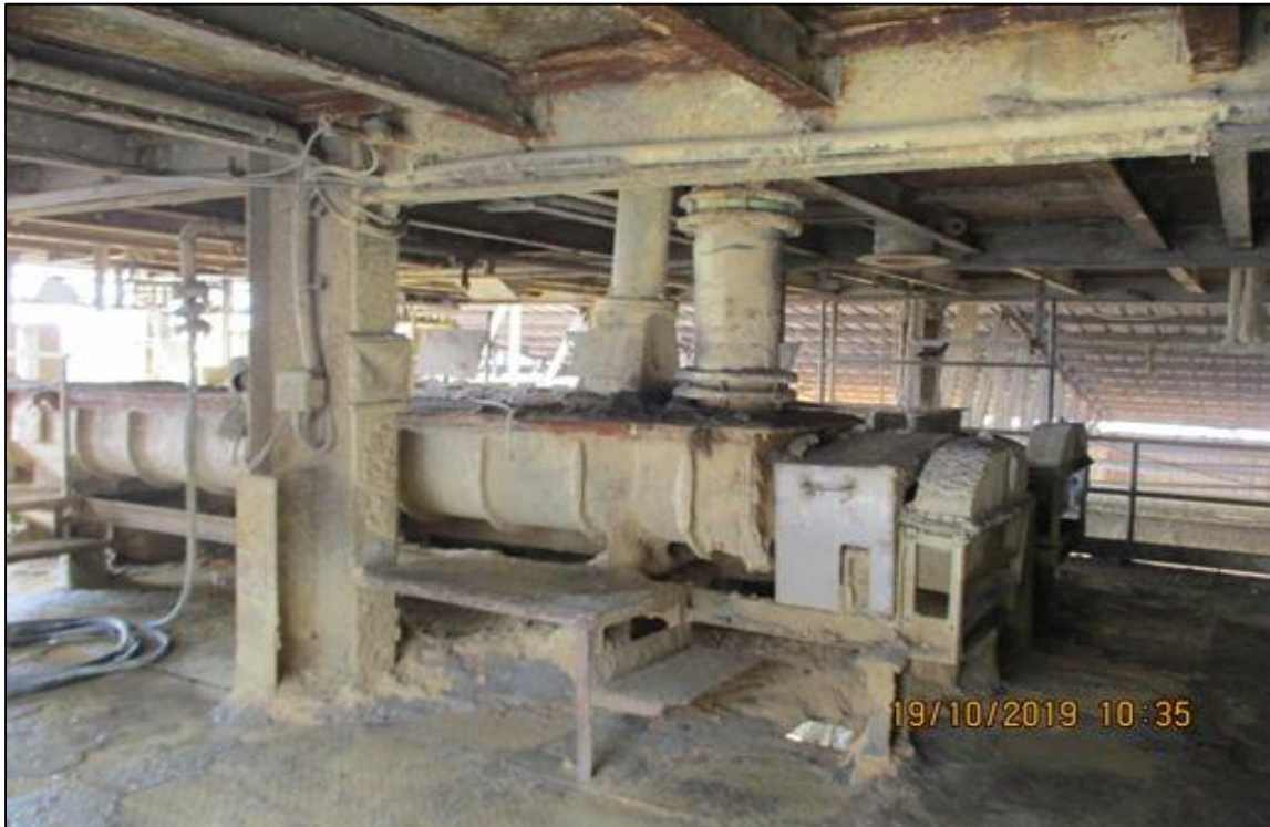
Figure 23: Cement mixer for Stabilized Jarosite at Chanderiya hydro smelter
