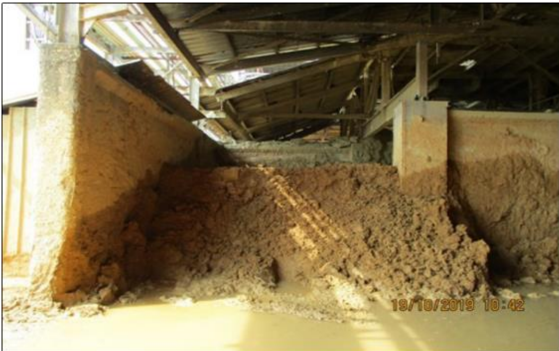
Figure 24: Stabilized Jarosite in curing yard after cement mixing at Chanderiya hydro smelter
