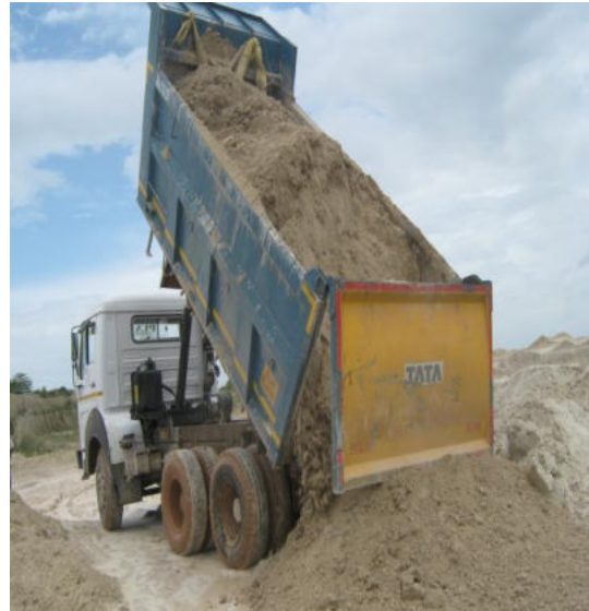
FIG. 5 & 6. Truck loaded with phosphogypsum in Phosphoric Acid plant and unloading in phosphogypsum stack area (Dry stacking)
