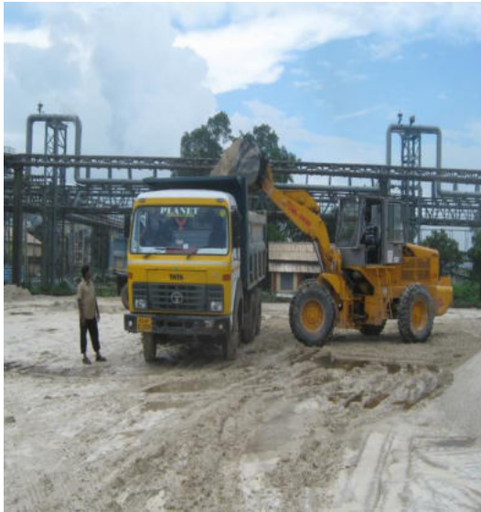
FIG. 5 & 6. Truck loaded with phosphogypsum in Phosphoric Acid plant and unloading in phosphogypsum stack area (Dry stacking)
