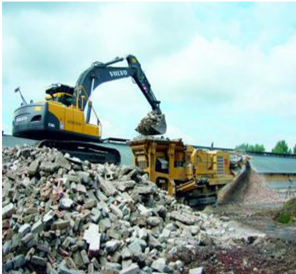
Crushing units at Burari C&D waste recycling plant Picture credits: IL&FS Pvt Ltd
