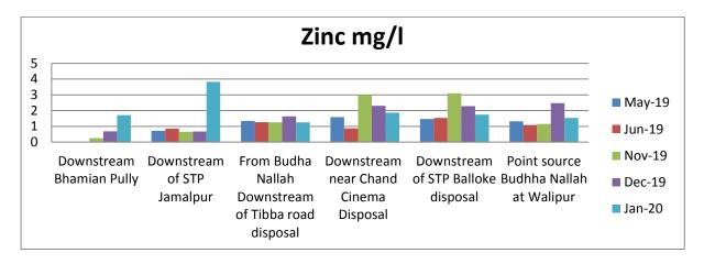
It has been observed that the concentration of Zinc has increased at the downstream of STP Jamalpur& downstream of Chand Cinema disposal.
