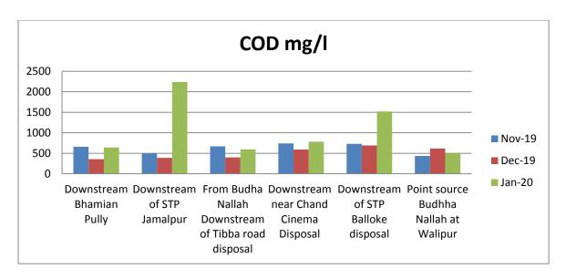
It has been observed that the concentration of COD has increased at the downstream of STP Jamalpur, downstream of Chand Cinema disposal & STP Balloke.
