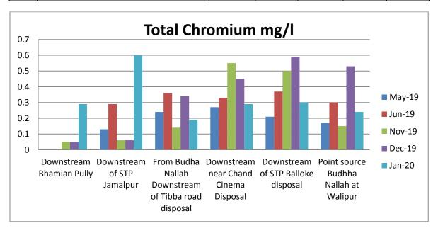
It has been observed that the concentration of Total Chromium has increased at the downstream of STP Jamalpur, downstream of Chand Cinema disposal & STP Balloke.
