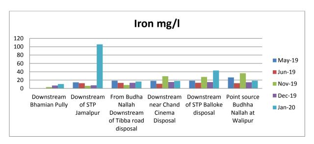
It has been observed that the concentration of Iron has increased at the downstream of STP Jamalpur& STP Balloke.
