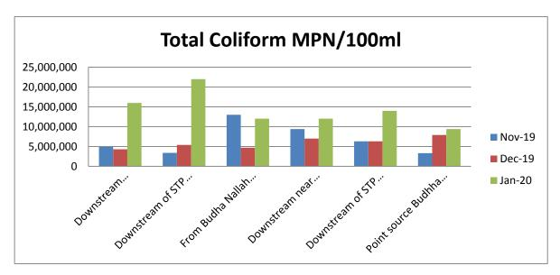
It has been observed that the concentration of T. Coli is already high at the downstream of Bhamian Pully and has further increased at the downstream of STP Jamalpur. Increased trend of T. Coli has also been observed at the downstream of STP Balloke.
