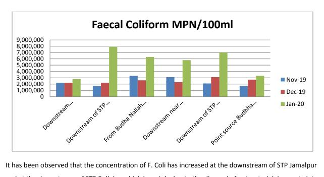
It has been observed that the concentration of F. Coli has increased at the downstream of STP Jamalpur and at the downstream of STP Balloke, which is mainly due to the disposal of untreated dairy waste into Budha Nallah.
