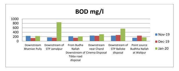
It has been observed that the concentration of BOD has increased at the downstream of STP Jamalpur, downstream of Chand Cinema disposal & STP Balloke.
