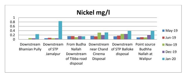
It has been observed that the concentration of Nickle has increased at the downstream of STP Jamalpur, downstream of Chand Cinema disposal & STP Balloke.
