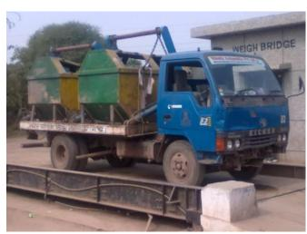
In processing plant, firstly the received waste weighed on Weigh Bridge of 25 ton capacity. Records of received waste maintained regularly. Received waste contains 30% inert, 20-25% Refuse-derived fuel (RDF), 15% compost & 35% inorganic. Plastics, rubbers,
