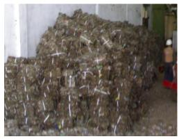
Refused derived fuel (RDF) contains 4-5% of 7,000-8,000 Calorific values plastics, 90% paper, organic matters and woods etc. Samples of RDF send to in house laboratory to calculate calorific value. The flow chart of RDF preparation is given at *Annexure* – *II.* The each packet of RDF has
