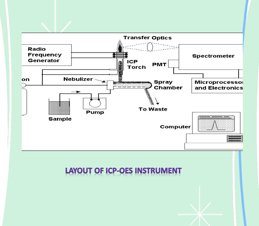
INDUCTIVELY COUPLED PLASMA **OPTICAL EMISSION** SPECTROMETER SPECTRON **INDUCTIVELY COUPLING:** Process of transferring energy to a system through the use of electromotive forces generated by magnetic fields.
