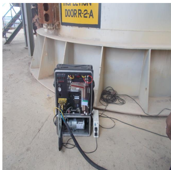
Arrangement made for monitoring source emission during pre trail, trail and post trail run of co-processing
