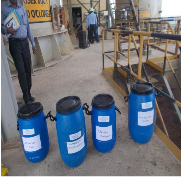
Arrangement made for composite sample collection of ETP sludge, Lime stone, clinker and fuel
