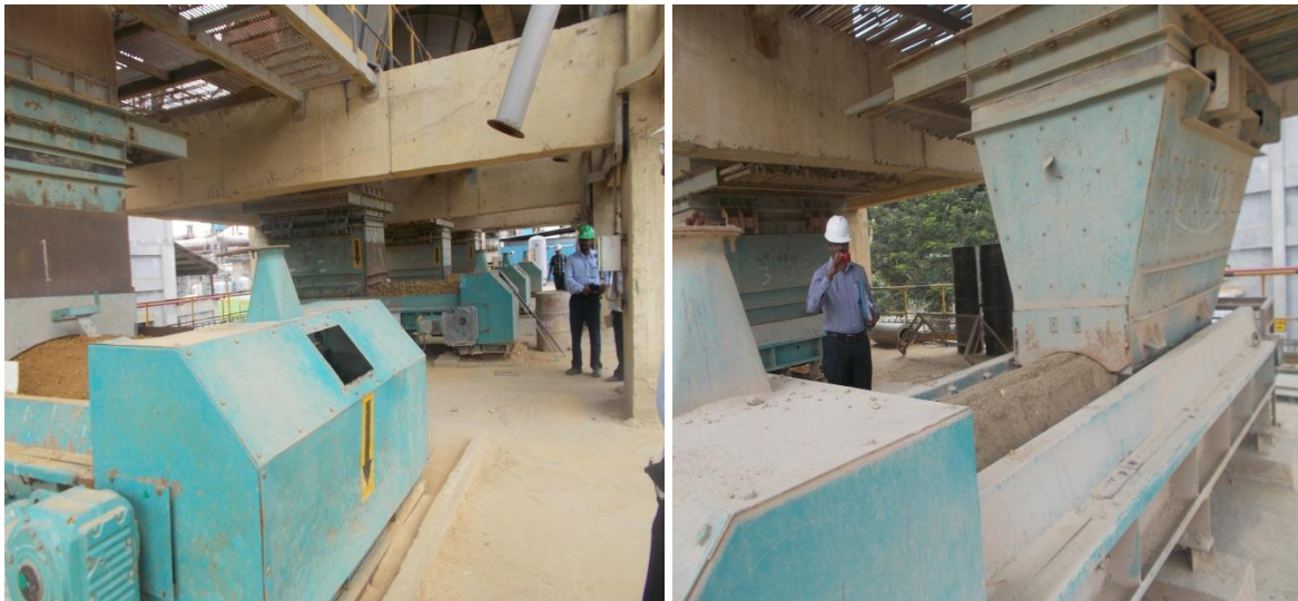
4 belt conveyor with hopper for feeding raw material to kiln in which one is dedicated for feeding ETP sludge
