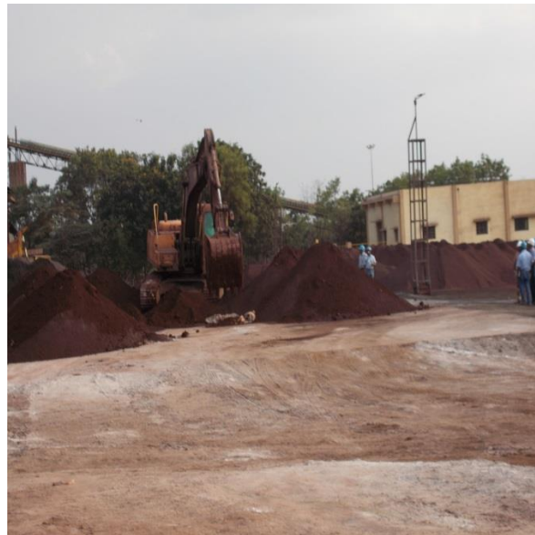
Mixing of Iron Oxide & Iron Ore fine
