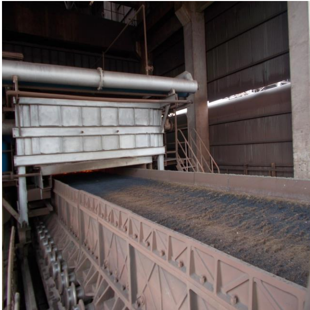
Sinter Plant -1 where Iron Oxide was utilised as supplementary raw material
