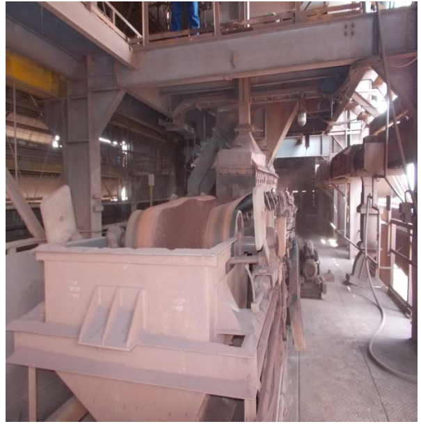
Feeding of Blended raw material into Sinter Plant 1
