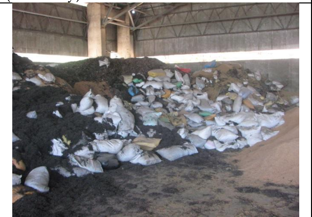
Fig.6: Alternate fuels stored in a shed
