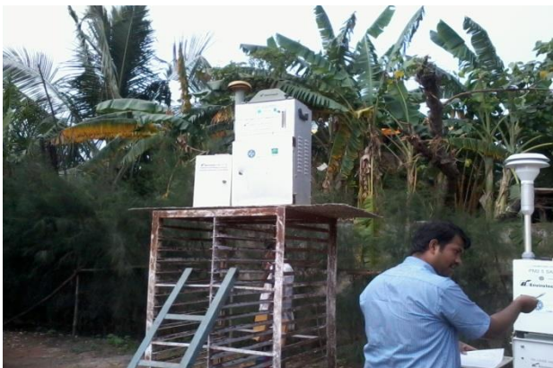
Plate 3. Ambient Air Quality Monitoring at North West (NW) corner (Workers Quarters)
