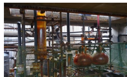
Fig 43 : Bromine recovery fro HBr Solution
