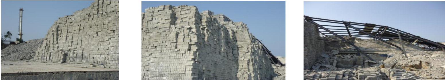
Fig 70: The Barite Mud Sludge made into Bricks and stored in the premises
