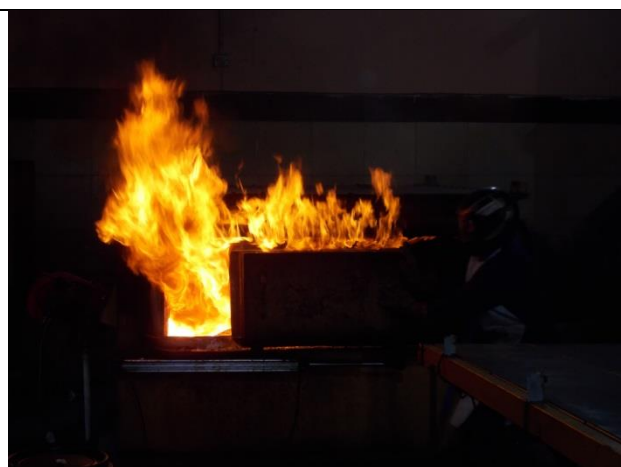
Fig.9: Negative draft is not maintained at primary combustion chamber, emission during charging.
