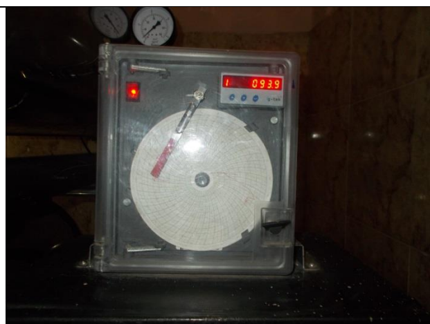
Fig.15: Autoclave temperature recording chart, where batch number, date are not mentioned.
