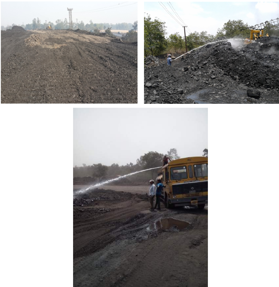
Fig-5.8: Fire fighting at coal stockyard and compaction of stock to prevent fire
