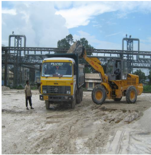
Figure 6 & 7: Phosphogypsum loading to truck in phosphoric acid plant and unloading in phosphogypsum stack area (Dry stacking)
