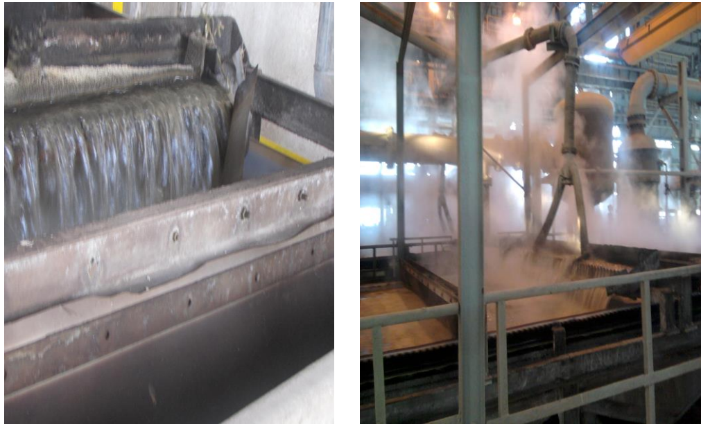
Figure 3: Washing of phosphogypsum prior to the storage or disposal
