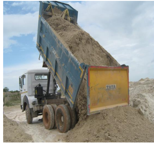
Figure 6 & 7: Phosphogypsum loading to truck in phosphoric acid plant and unloading in phosphogypsum stack area (Dry stacking)
