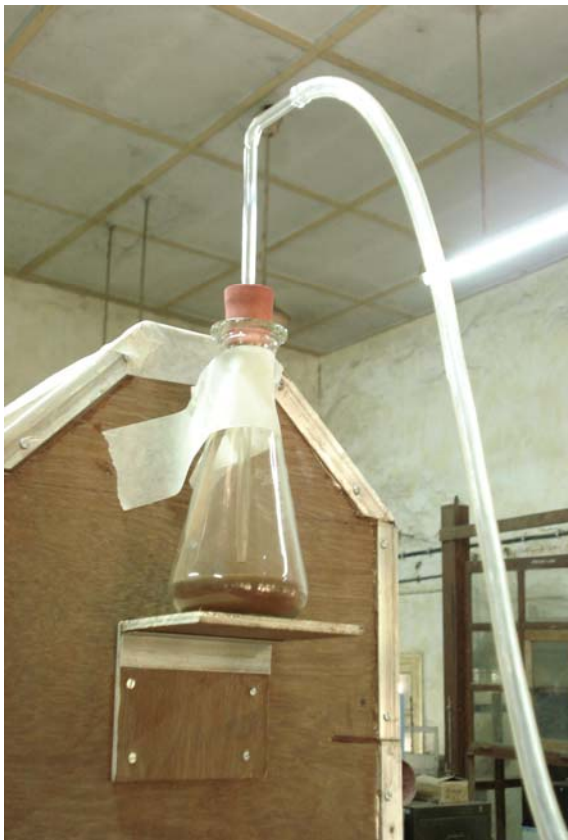
Figure 3.4 : Laboratory setup for the Resuspended Dust Chamber
