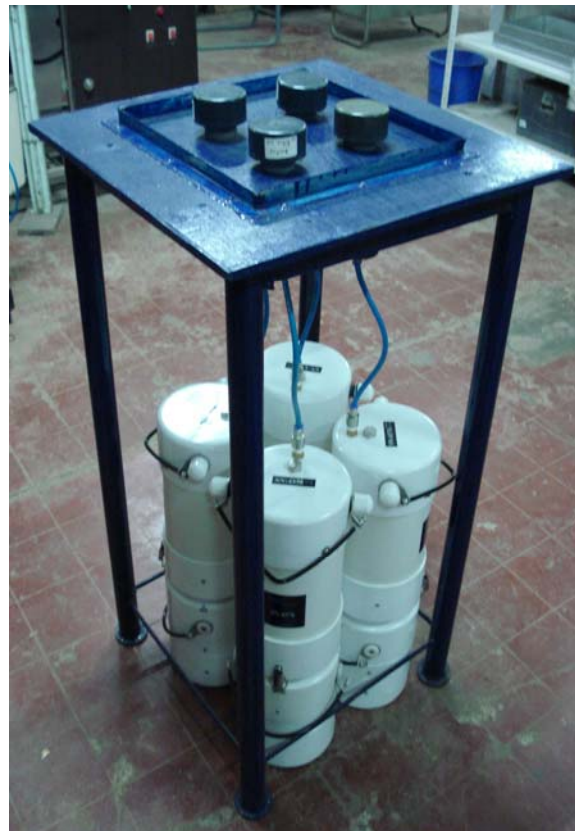
Figure 3.4 : Laboratory setup for the Resuspended Dust Chamber
