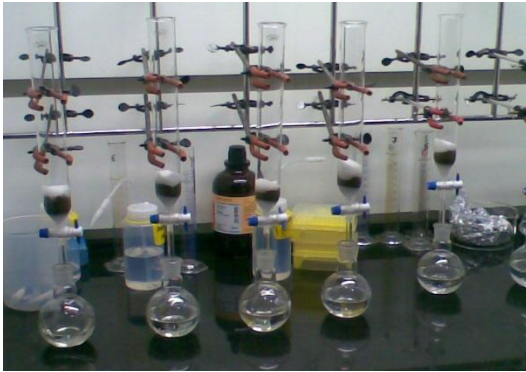
Extract Columns Clean-up Assembly
