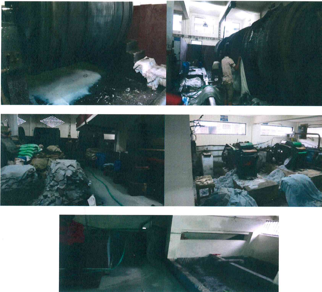
Poor Housekeeping resulting the spread of industrial effluent on the floor
