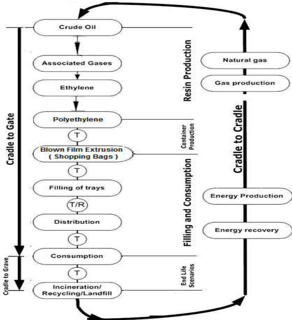
Figure 10: Flow chart for LCA of HDPE bag process
