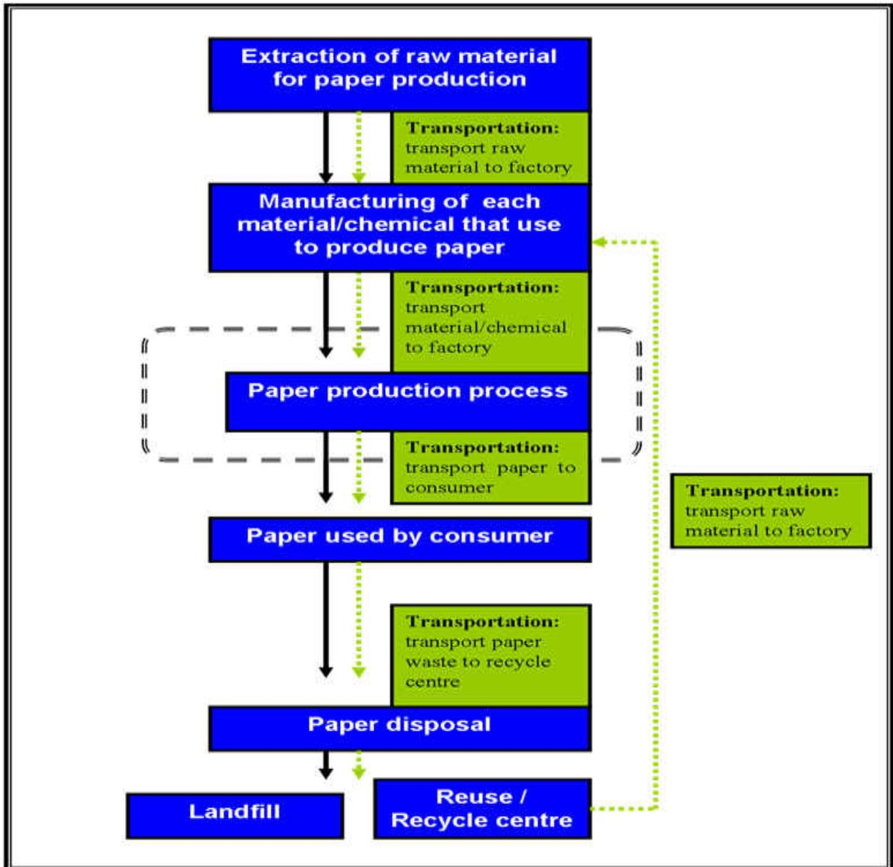
Figure 9: Flow chart for LCA of paper bag process
