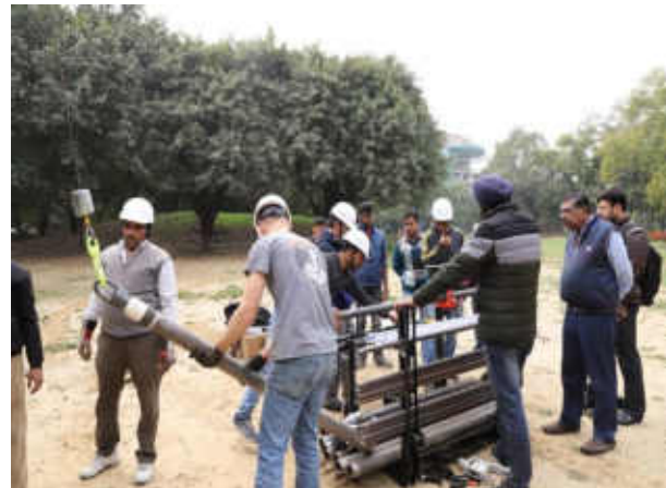
f. Raising of outer casing (probe rod) for direct push sampling
