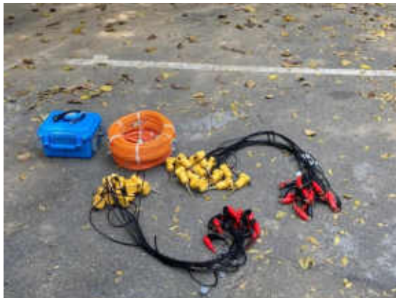
(a) MASW Instrumentation
