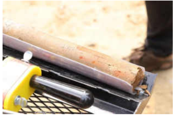
j. PVC liner cut open to extract specimen for laboratory testing
