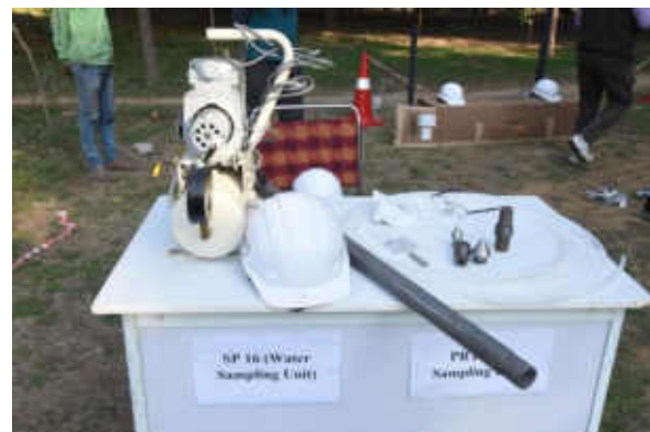
(c) Groundwater Sampling and Pore-Gas Vapour Sampling Units
