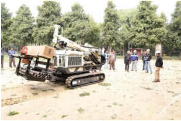
c. Environmental soil sampling rig with mast in folded position
