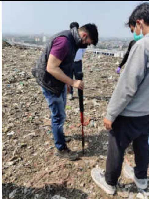
(a) Installing Gas Vapour Probe at MSW Dumpsite
