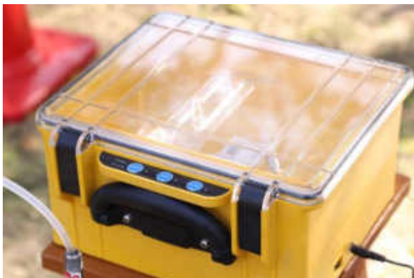
(g) Automatic Vacuum Gas Sampling Box
