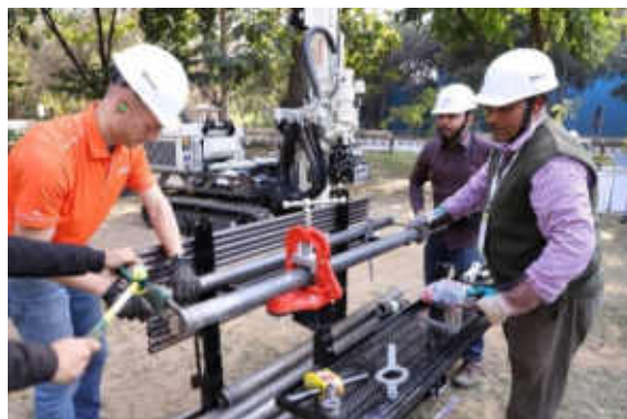
(g) Removing Liner from the Inner Tube
