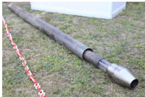
(b) A Typical Dual Tube with Liner and Cutting Shoe
