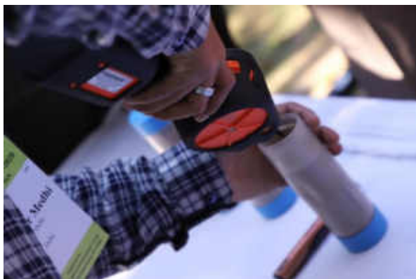
(c) Samples being checked for VOCs
