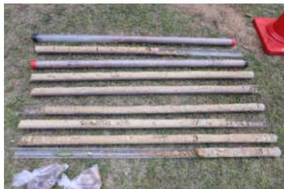
(h) Liners Containing Continuous Core Samples
