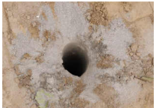
n. Borehole (15 m deep) after completion of direct push sampling
