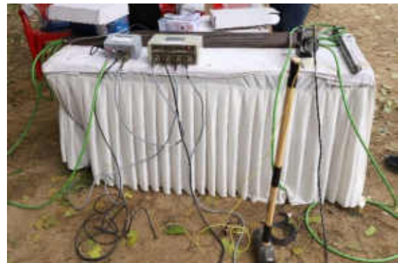
(h) Connecting Cone, CPT Controller and Laptop
