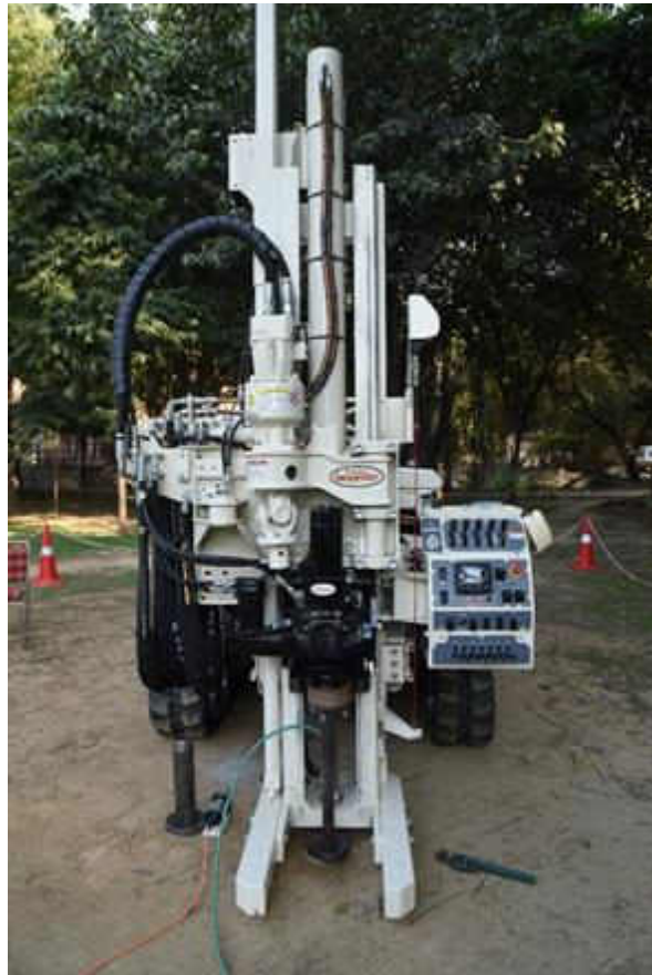
(a) The Geoprobe 7822DT Drill Rig
