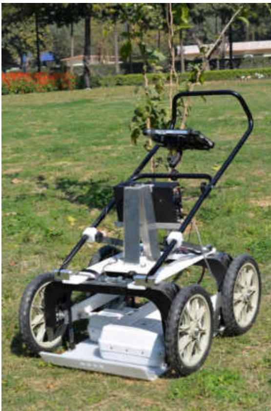
(a) Ground Penetration Radar Assembly
