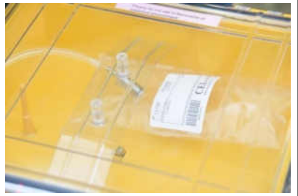
(h) Gas Sampling in a Tedlar Bag in the Sampling Box
