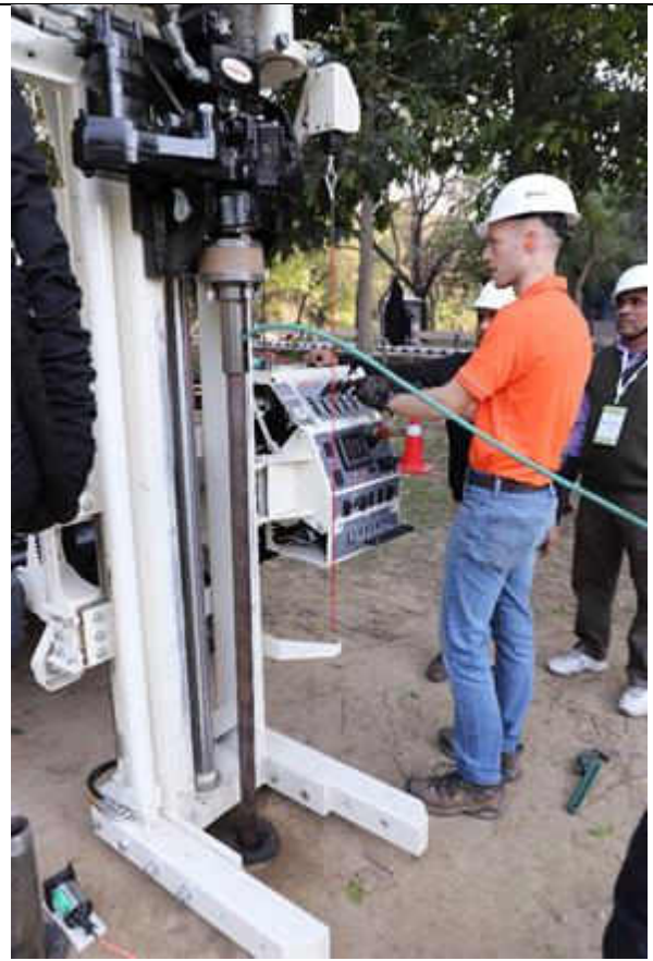
(f) Performing OIHPT test
