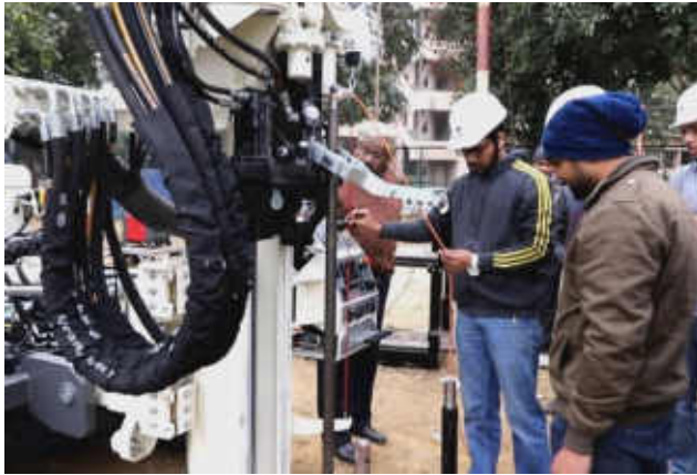
(m) Pulling Out Rods and Cone
