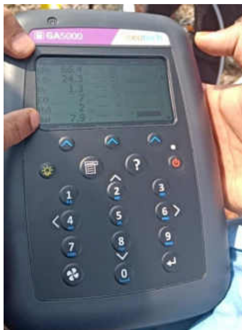
(b) Recording Concentrations of Landfill Gas Constituents
