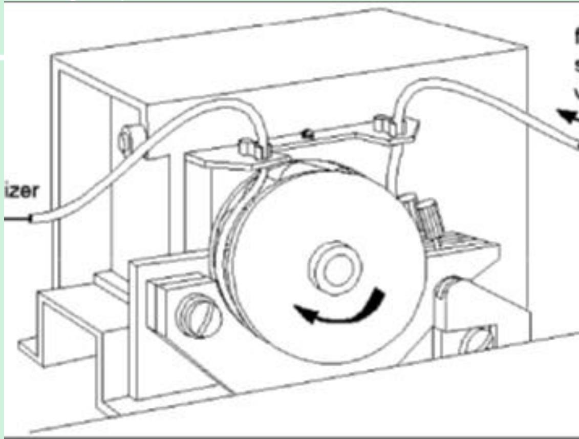
PERISTALTIC PUMP USED FOR ICP-OES
