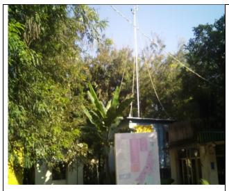
Lot of trees grown up around the CAAQMS at IITM, Chennai and obstructing the free flow of air which resulting in non-representative of the concentration measured
