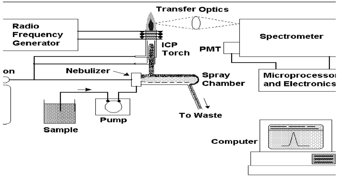
**LAYOUT OF ICP-OES INSTRUMENT**
