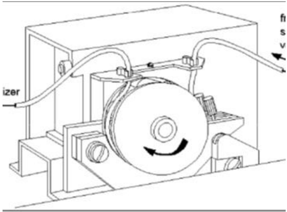
**PERISTALTIC PUMP USED FOR ICP-OES**
