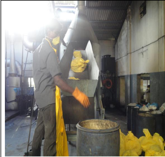
Fig.7: Loading of Bio-Medical Waste in Conveyor system
