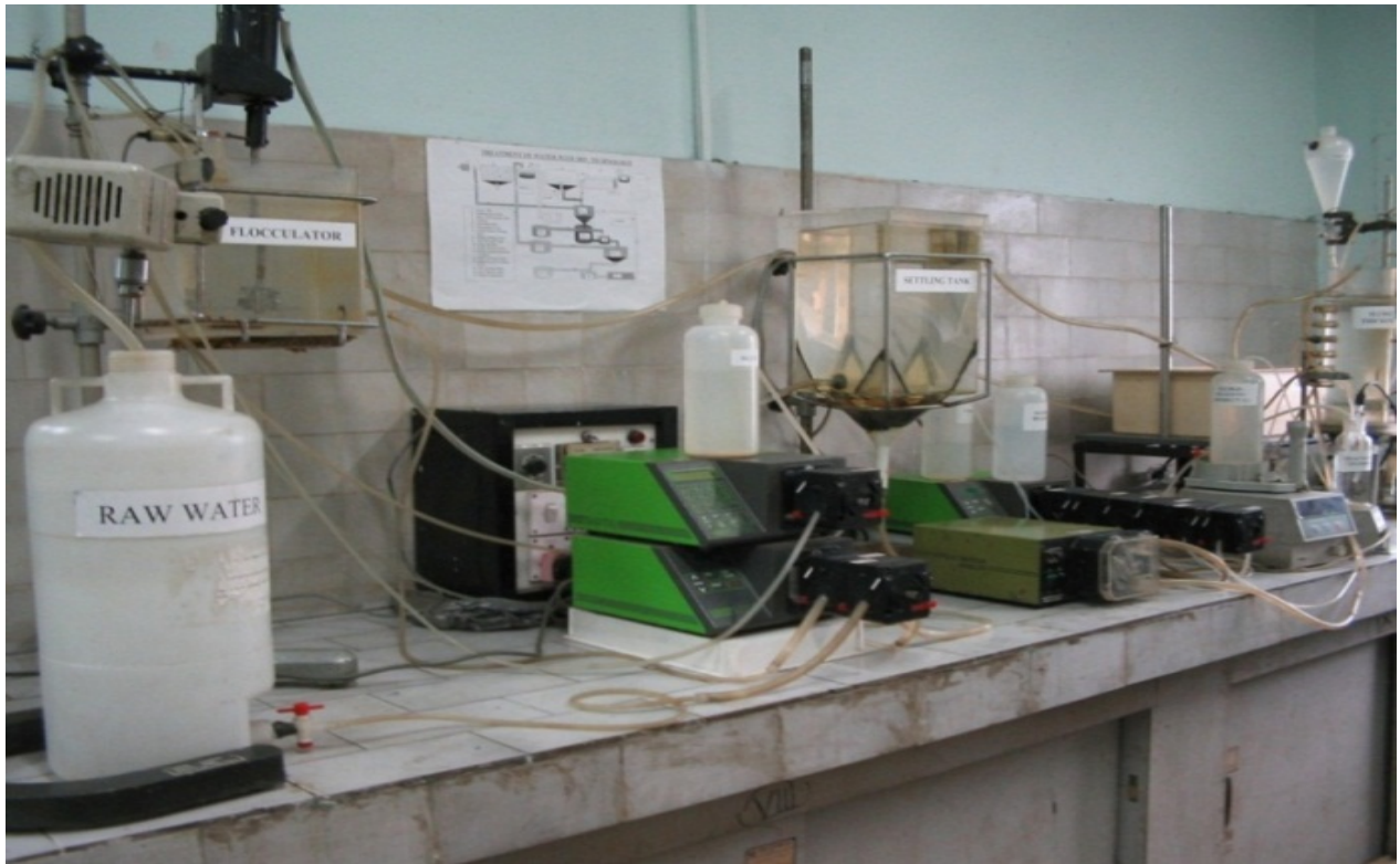
LABORATORY SCALE WORKING MODEL OF SRP BASED TREATMENT TECHNOLOGY
