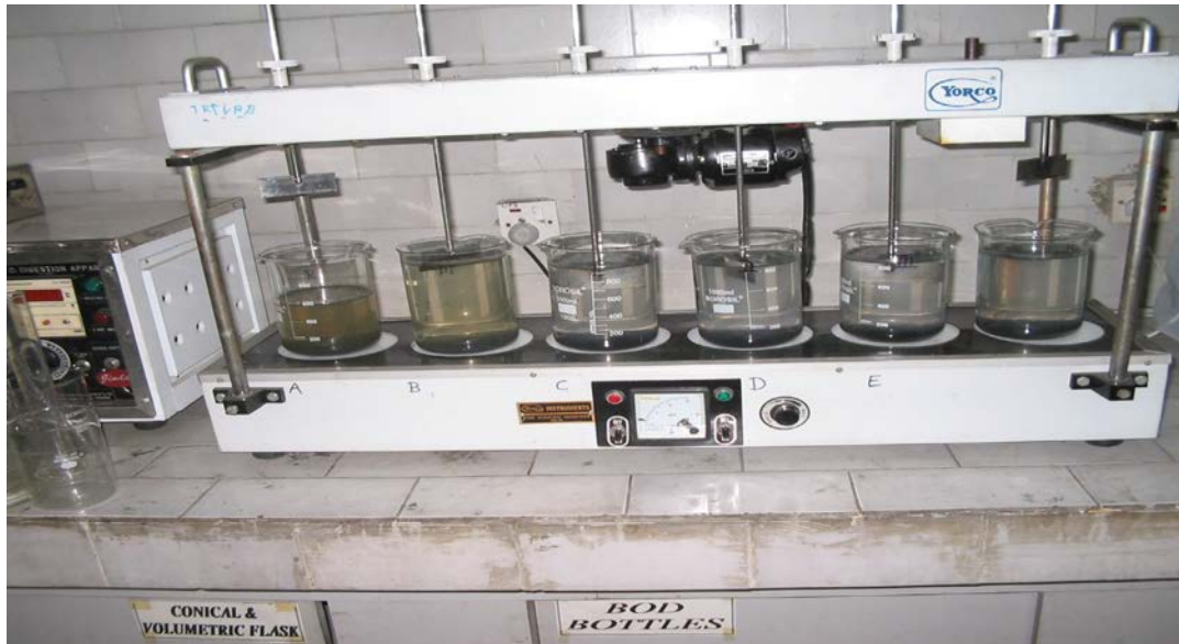
Figure -3 shows : Alum dose optimization , using Jar Test Apparatus.
