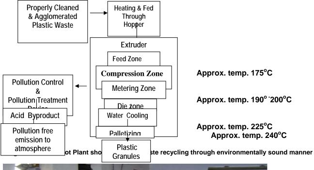
Process Flow-Chart of the "Green Recycling Process" - The Pilot Plant
