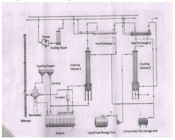
Figure 3 : Schematic flow-diagram of conversion of plastic waste into liquid fuel (RDF)
