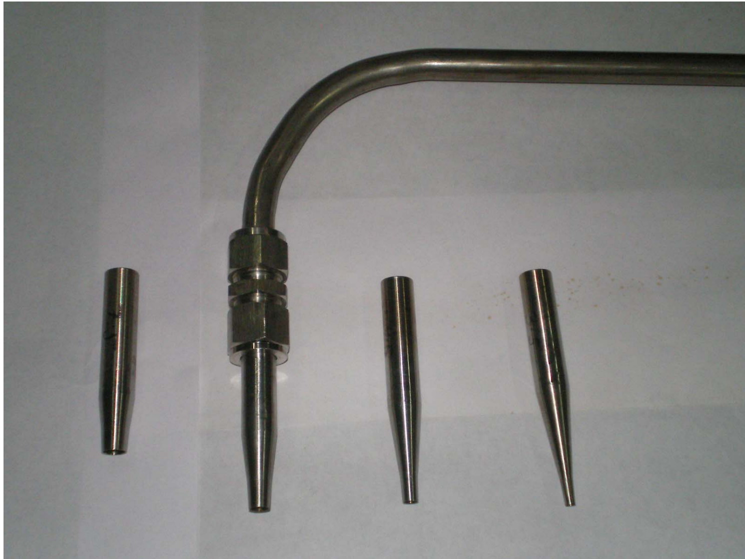
Figure 3.2 Photograph of iso-kinetic sampling probe with interchangeable nozzles.
