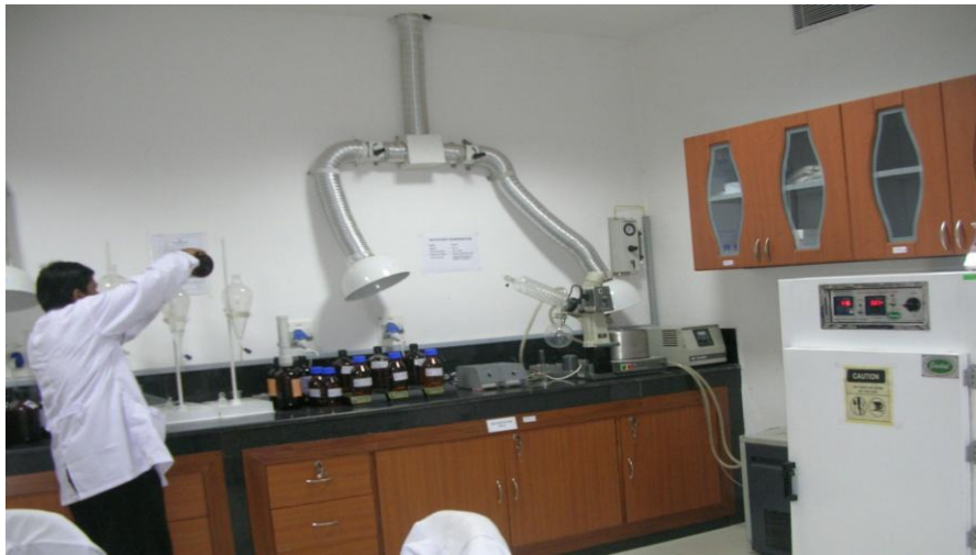
Pesticides Samples Liquid - Liquid Extraction
