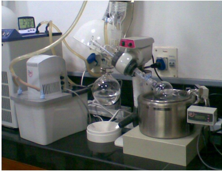
Eyela (Japan) Rotary Evaporator with Vacuum Pump and Recirculating Chiller
