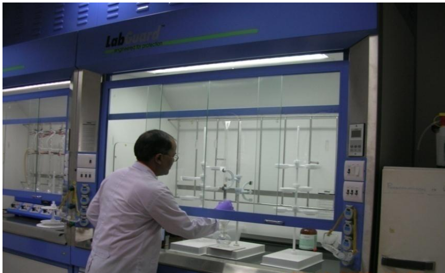
Sample Processing & Pre-Treatment Fume Hoods
